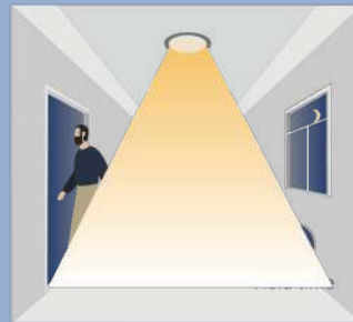
Light goes to the holdtime and keeps current brightness after motion leaves.
