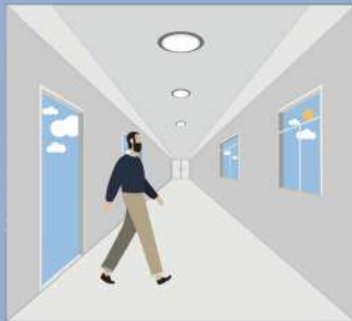
With sufficient daylight, even when motion detected, light remains OFF.
